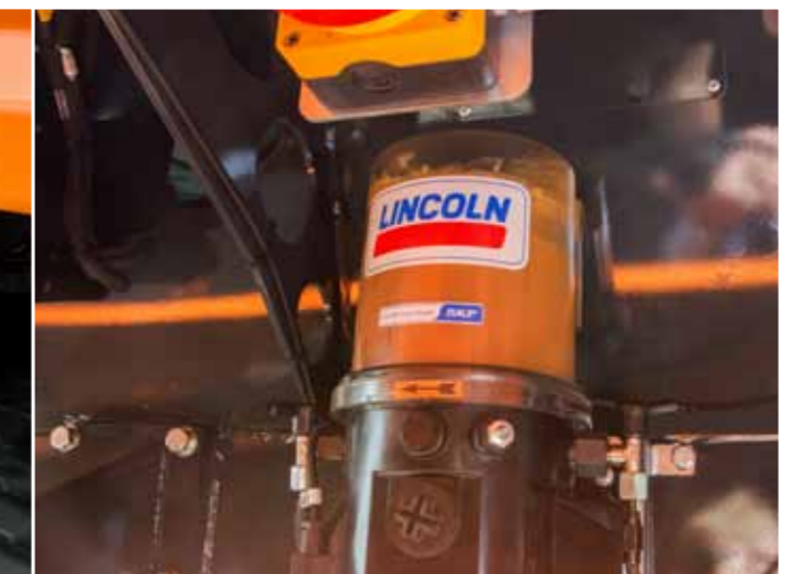
Central lubrication system Provides automatic lubrication of all key machine components.
