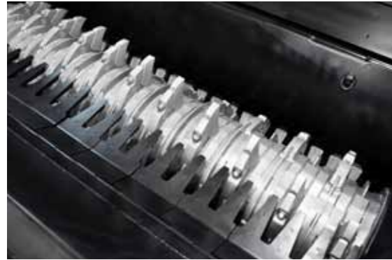
Single shaft with max. 27 rpm. Depending on the input material different types of knives are available: breakers (for wood, green waste, household, plastic), cutting (for rubber, foil, plastics, fabrics) and crumbling (for roots, logs, railway sleepers)
