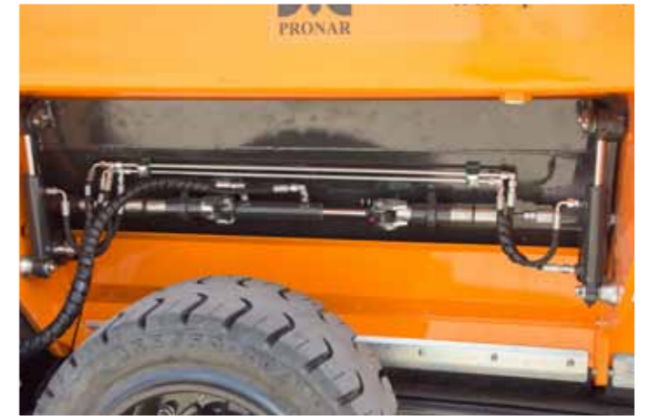
Hydraulic side combs. Set fraction size of crushed material in matter of seconds without any tools.
