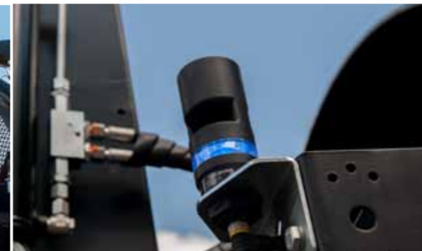
Beacon light signalises work/drive mode
