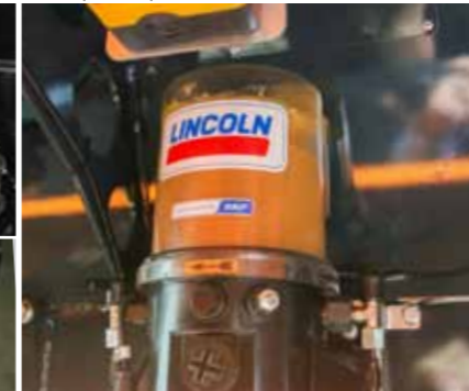
Central lubrication system ensures good greasing of most importants parts of the machine
