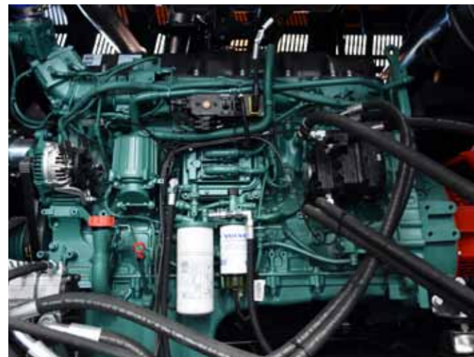
Engine - Voivlo Penta (550 hp/ 405 kW)
