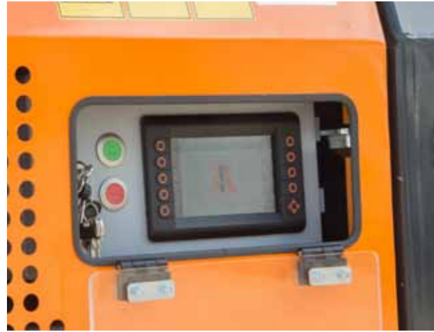
Easy to use touch-screen control panel to set all important functions of the machine.
