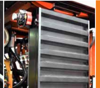
Cleanfix systems automatically clean engine and oil hydraulics radiators
