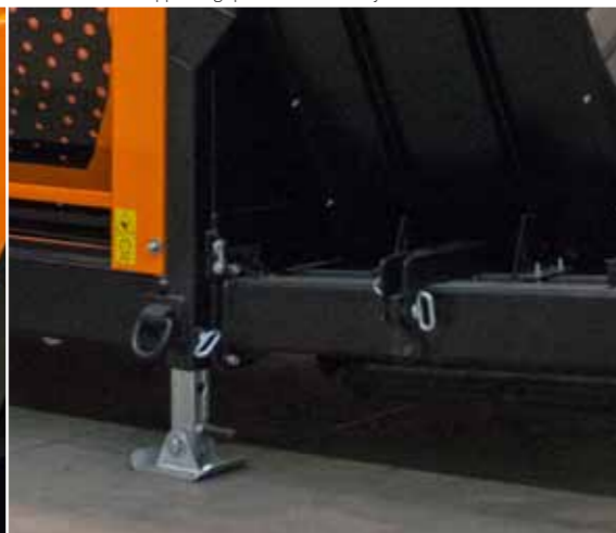
Mechanical front support legs provide the stability of the trommel
