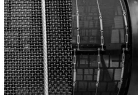
Steel lifters in the drum help more efficient separation and screening
