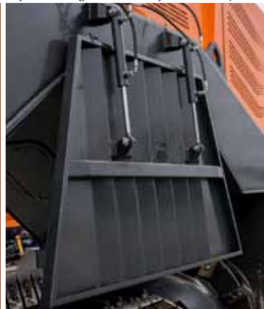
Adjustable tailgate limits the ejection of compost
