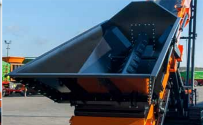
The beam with adjustable dampers relieves the belt and eliminates dynamic loads during feeding
