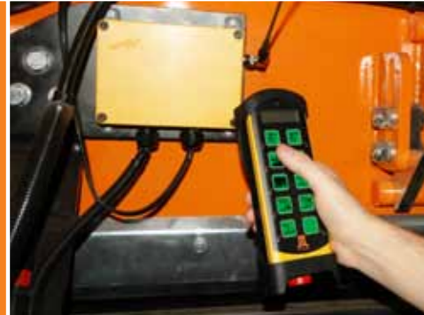
Remote control for basic machine operating functions
