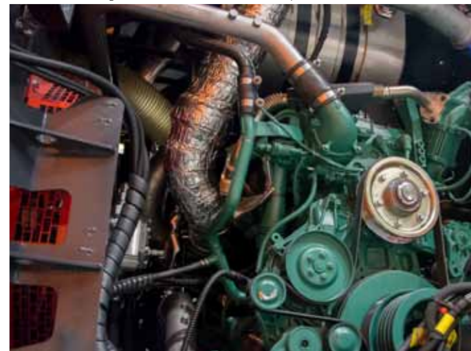
Engine Volvo Penta (EU Stage V, 13L, 390 kW, 530 BHP @ 1900 rpm)
