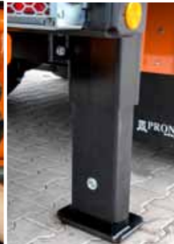
Hydraulic support legs ensures stability of machine
